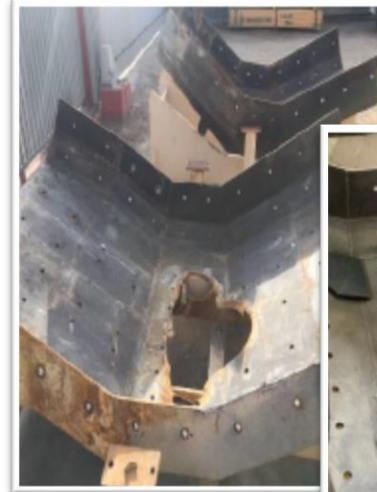
Repair Motherboard and ceramic coating Deflector
