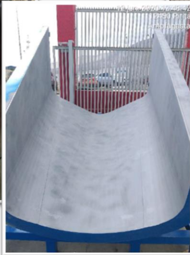
Manufacturing and Coating Silicium carbide Sealing Slide
