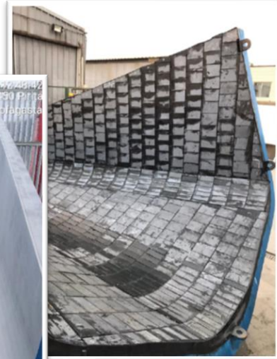
Manufacturing and Coating Silicium carbide Sealing Slide
